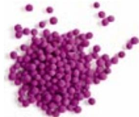
In addition to the active oxidation effects, the purple colour is part of innovative "ENTEC Consumption indication system". The colour change that occurs during operation serves as a visual indicator that indicates the consumption level of the product at all times.
