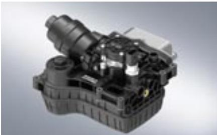
In addition, the system has moisture, pressure and temperature sensors, a switchable electric pump and an oil cooler with optional thermostat control. An oil dryer is part of the oil filter system and constantly maintains the oil quality at a high level and efficiently separates any water which has dissolved in the cooling oil. The highly efficient adsorber material of the oil dryer removes even the smallest amount of water from the oil.
